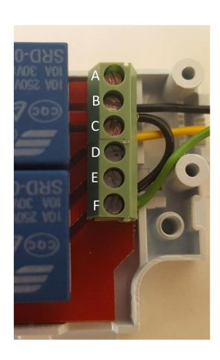
The relays terminals are used to connect and disconnect 2 circuits
