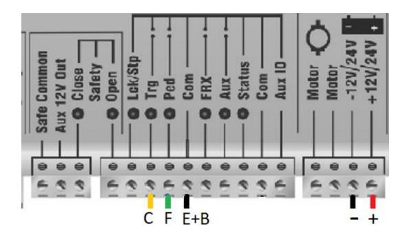
Connect the 2 common terminals together Connect terminal C to the TRG terminal Connect terminal F to the PED terminal
