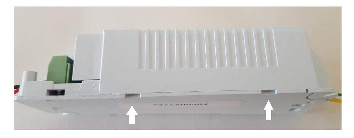
Ease a flat screwdriver into the slots on the cover and gently ease the cover upwards.
